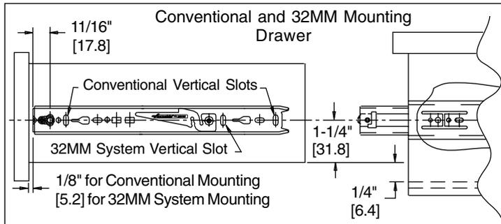
4. Make sure the ball bearing retainers in the cabinet side are fully forward. Install drawer into cabinet. Close the drawer.
